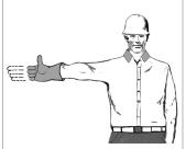
With arm extended horizontally to the side and thumb pointing up, fingers open and close while load movement is desired.
